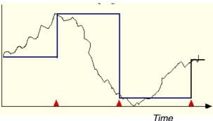
If the samples are not taken very often (where the red triangles are) then when the signal is converted back (the blue line) it only very roughly shows the shape of the original signal.
