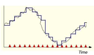
How often sampling is done therefore depends on the quality needed. For example sampling on a telephone landline is only 8000 times per second, that is OK for voices although they do sound a little distorted.
