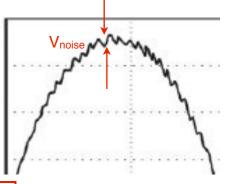
Max bits per sample  $b = log_2 \frac{V_{total}}{V_{noise}}$
