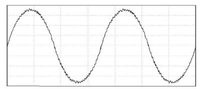
If the samples of this signal have a high definition, in other words there are lots of possible levels because there are a large number of bits per sample then all we will do is reproduce the noise. There is no point in that so we may as well send fewer bits per sample and save on the quantity of information sent.
