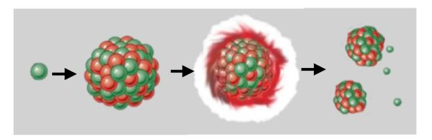
Nuclear Fission is the splitting of the nucleus of an atom into two or more parts by hitting it with a small particle, almost always a neutron (a proton would be repelled from the positive nucleus and an electron would have too little energy).
