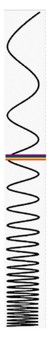
Radio waves roughly from up to 100Km down to a 10 mm wavelength produced by electrons oscillating in a conductor (a wire) used for message and music transmission. Shorter radio waves used for television signals.
